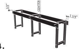
With the legs on a flat surface, fasten (2) 1x4's with 1" screws, as noted above. Leave a 1 1/4" overhang on each side, and offset 1/2" lower from the top of the legs.
