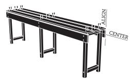
Align the remaining (3) 1x4's as shown above. The outside pieces should sit flush with the face pieces that were fastened in Step 4. Center the middle piece. Fasten with 1" screws at the top of each assembled leg.
