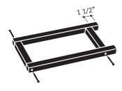
Assembling the legs: On a flat surface, align (2) 18" 2x2's with (2) 8" pieces as shown. Fasten with 2-1/2" screws. Repeat to make a total of (3) legs.
